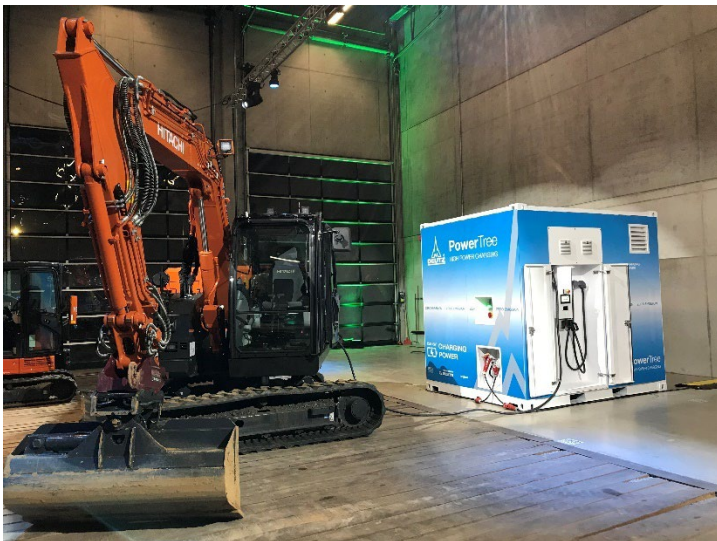
Picture caption: The DEUTZ PowerTree is an emission-free, on-site energy supply for electrical applications. Picture credit: DEUTZ AG
