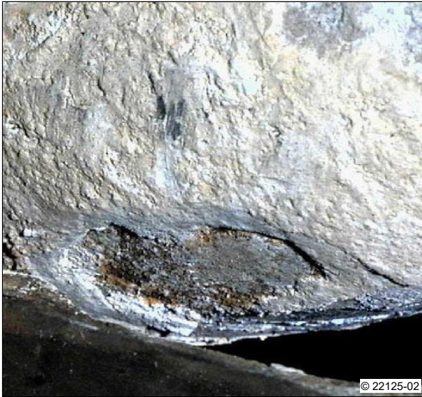
A13: Limescale deposits on a cylinder liner
