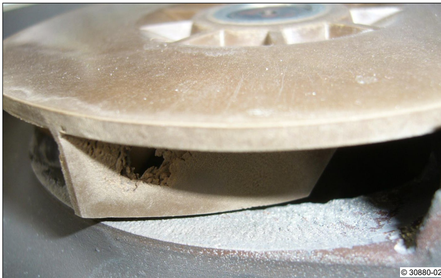
A15: Flywheel of the coolant pump, cavitated
