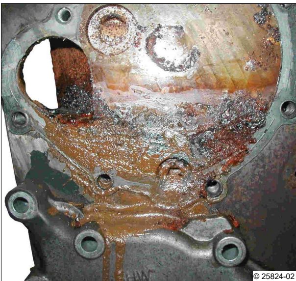
A9: Coolant pump seat on the crankcase
