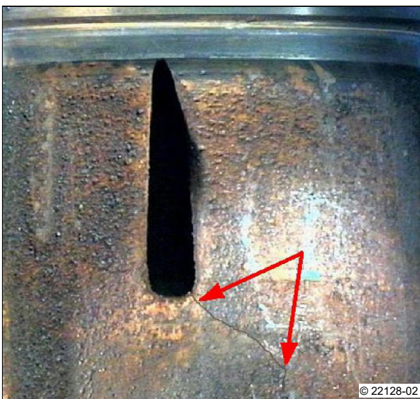
A3: Crankcase crack in the area of the cylinder liner
